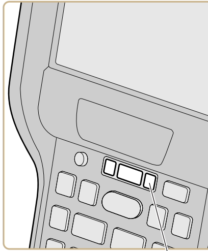
Battery status LED
